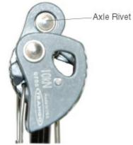
After receiving a defective unit from a climber in the field, in-house inspection and testing has revealed that a small number of our # 1 MaxCams have head axle rivets that do not meet the minimum specified diameter, possibly resulting in failure of the cam assembly. This flaw affects only the red #1 MaxCam with Batch Numbers 0605 and 0705 that were sold in 2005 and 2006. All other cams are unaffected and you can continue to use them with confidence.
